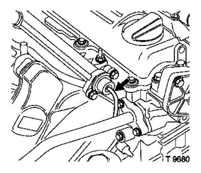
Fuel distribution pipe from the intake manifold.
