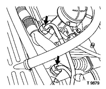
Ground cable to the engine control unit - bolt (2).
