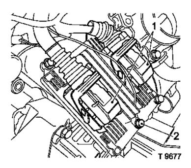
Wiring harness connector to injectors.
