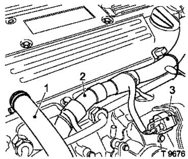
Wiring harness connector (1) from the engine control unit.
